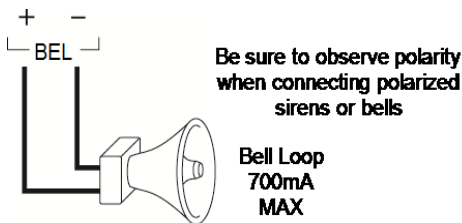
Figure 1-5 Bell Wiring
